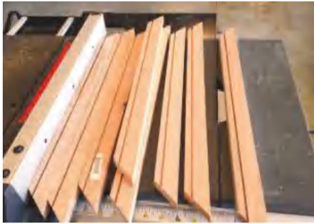
STEP 19. Measure and cut the front doors with a 45° angle. Rip and notch the door frame pieces to allow for the plexiglass insert
